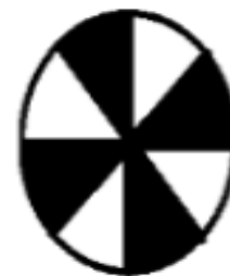
Fig. 1 Bi-colour slot encoder disc
